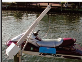
PWC DAVITS LIFTING HARNES AND PWC LIFTS
