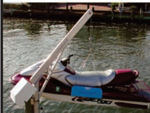
PWC DAVITS LIFTING HARNES AND PWC LIFTS
