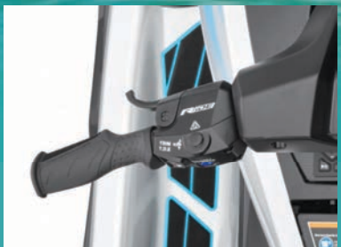
SWITCH FROM NEUTRAL TO REVERSE WITH ONE PULL OF THE THROTTLE
